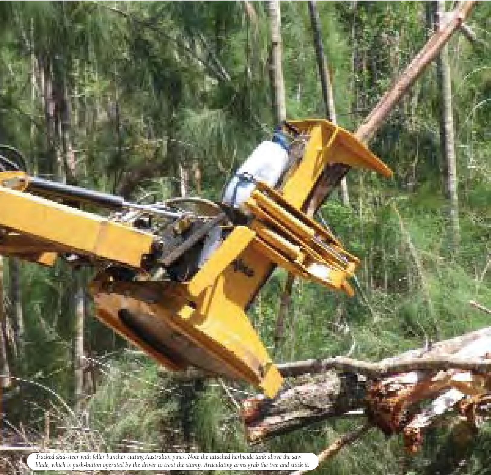
Tracked skid-steer with feller buncher cutting Australian pines. Note the attached herbicide tank above the saw blade, which is push-button operated by the driver to treat the stump. Articulating arms grab the tree and stack it.
