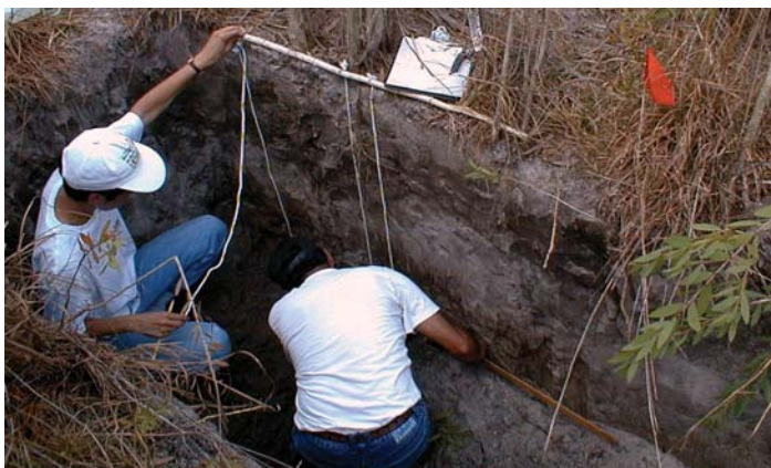
Photo 1. A soil trench method was used to measure the root distribution and density of field grown Melaleuca quinquenervia trees in an age sequence.
